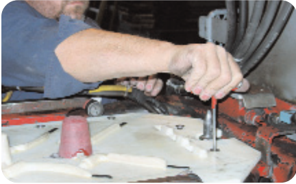
Figure 9: The FDM matchplate is mounted to the automatic molding machine's pattern frame.
