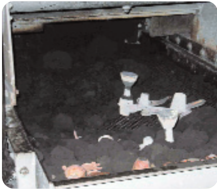
Figure 14: Raw casting surrounded by loose sand after the vibratory process.
