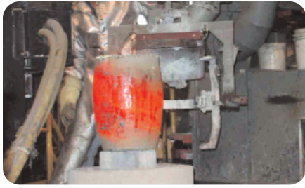
Figure 13: Crucible, filled with molten bronze, just prior to pouring into the mold.
