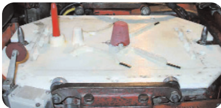
Figure 2: FDM matchplate, mounted in automatic molding machine, can withstand the ramming forces used to pack sand casting tools.
