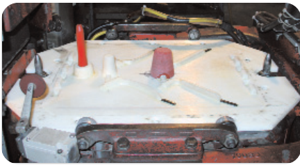
Figure 8: FDM matchplate made in ABS with sprue attached.
