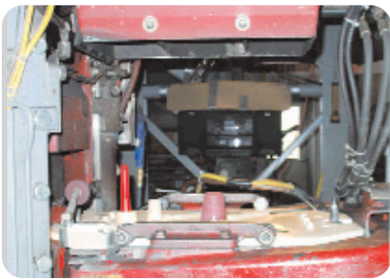
Figure 10: FDM matchplate is raised and mated with the flask for packing the sand casting tool.
