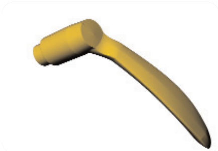
Figure 5: CAD file of door handle with draft and shrinkage allowance.
