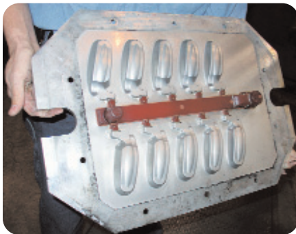
Figure 1: Machined aluminum matchplate.
