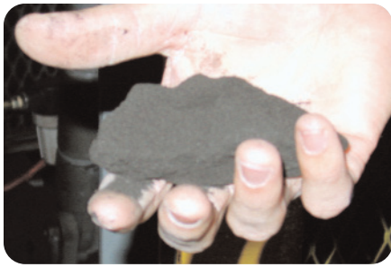
Figure 4: Green sand, as shown here, retains its shape when compacted.
