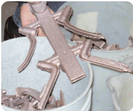
Figure 15: Raw bronze casting, with gates, runner, riser and sprue, is ready for machining.
