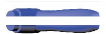
Figure 6: For split patterns, the CAD file is separated along the parting line.
