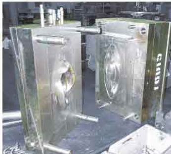
This injection-molding tool for one component was used during the engineering pilot.
