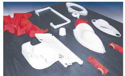
Shown are some of the 31 components prototyped on the Stratasys FDM Quantum.
