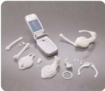
Image 1: Logitech’s mobile Bluetooth® headset in use. Image 2: Logitech redesigned its headset to improve the microphone boom’s strength. Image 3: Headset components were modeled in ABS plastic, using the FDM Vantage SE from Stratasys.
