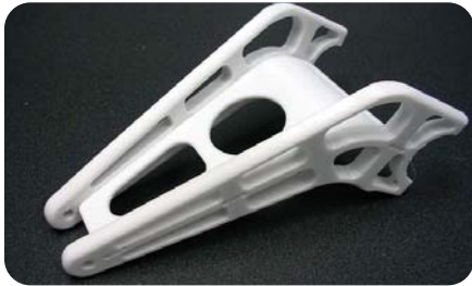
Images 4 & 5: CAD design and prototype of steering column bracket. This part would have required multiple setups if prototyped via CNC.
