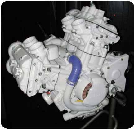
Image 1: The Desmosedici motorcycle. Image 2: The Desmosedici's engine was prototyped almost entirely from polycarbonate using FDM.
