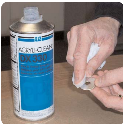
Figure 3: Degreasing metal insert.
