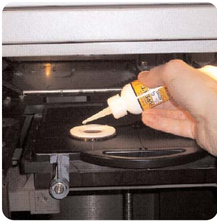
Figure 5: A few drops of super glue aids in preventing movement of the metal insert.
